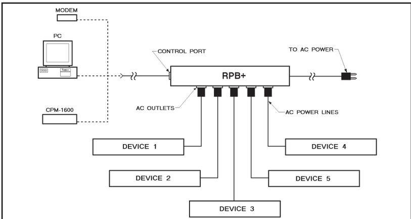
Figure 4: RPB+ Cable Connections
