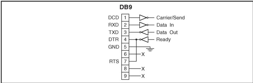
Figure 3: RS-232 (Control Port) Interface Schematic
