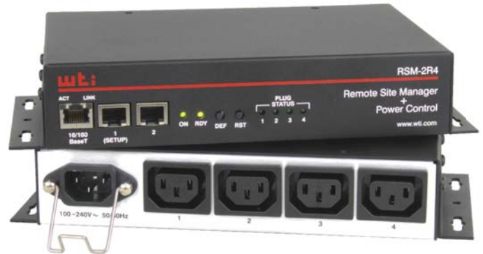
Model RSM-2R4-2F (4) IEC-60320-C13 Outlets + (2) Remote Console Ports
