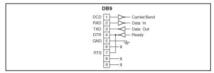
Figure 3: RS-232 (Control Port) Interface Schematic
