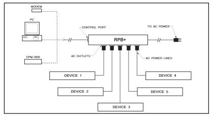
Figure 4: RPB+ Cable Connections
